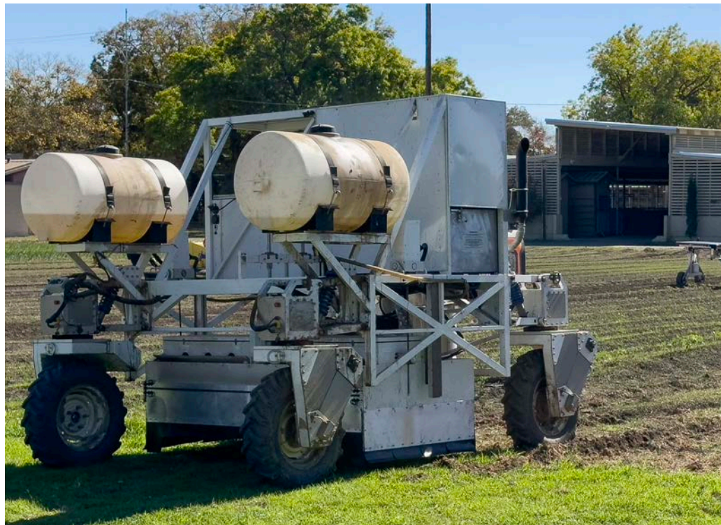
The weed-killing robot, Jetty, from Tensorfield Agriculture uses computer vision to identify weeds
