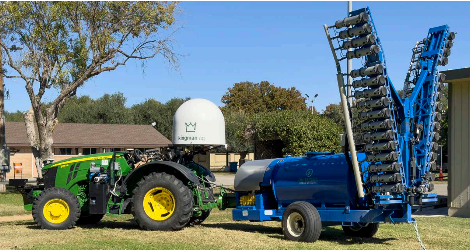
Many components are required for autonomy, including the JD Link modem, Starfire receiver, G5 display, and John Deere Operations
