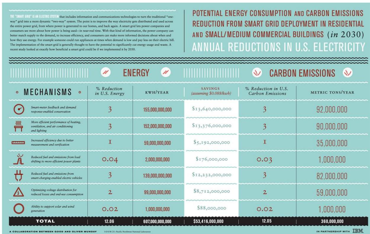
Direct tangible consumer cost savings are also an important factor. To reduce demand during the high cost peak usage periods, communications and metering technologies inform smart devices in the home and business when energy demand is high and track how much electricity is used and when it is used.
