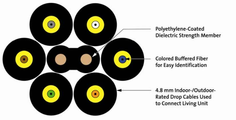
**Figure 2: Bundled drop cross-section**
