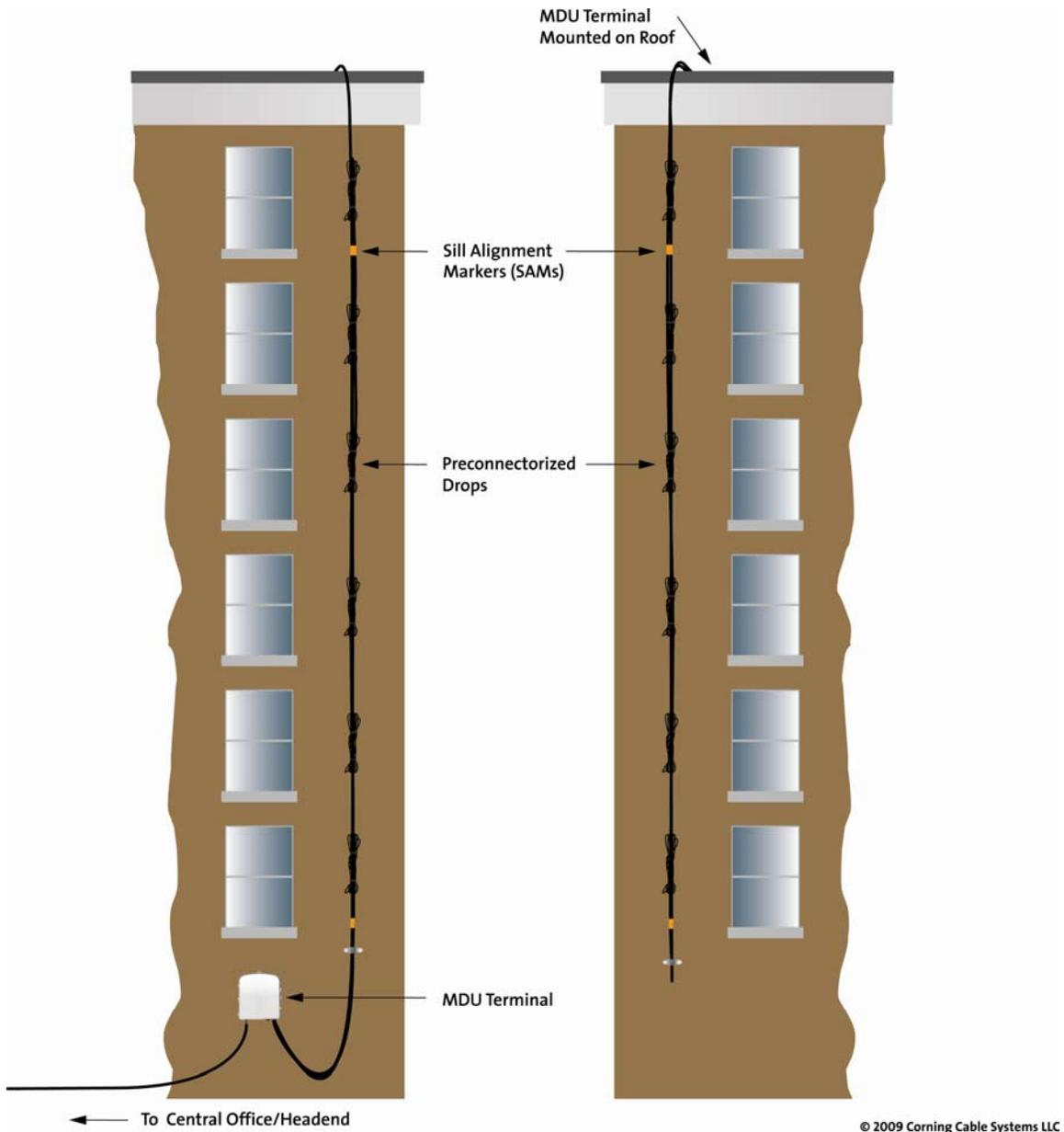
**Figure 1: Two deployment methods of bundled drop cable (feed-up and feed-down). (The cabling system is larger than scale for effect.)**
