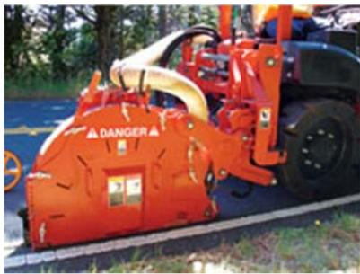
*The head of the trencher is the vacuum system mounted on a truck with a hose leading back to trenching component to remove spoil as the trench is cut.*
