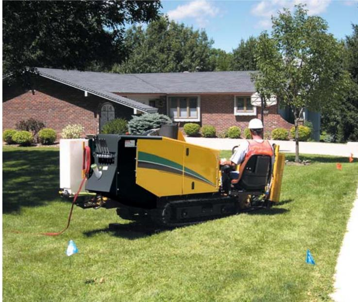
The HDD method is normally surface launched and is detected underground so operators can steer around obstacles. Steering allows operators the capability to maneuver around existing underground utilities. Another advantage of HDD is the ability to place the product deeper than a small plow, allowing the operator to place the new line under existing utilities.
