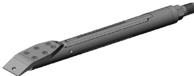
When pushing the drill head without rotation, the slanted bit causes the head to steer. If you rotate the drill head while pushing it forward, the head will follow a straight course.
