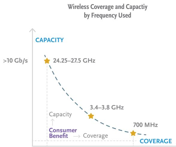
One of the limiting factors for 5G High-Band (whether used for mobile or residential use) is limited coverage. The Higher the 5G frequency, the higher the capacity for bandwidth (speed), but signal coverage is reduced dramatically—typically down to about an area about 650 feet in diameter.
