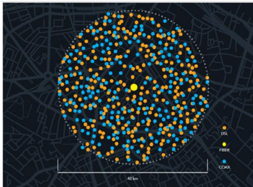
Typical powered equipment in a 40 Km area by provider type. FTTH has one powered point versus hundreds for other methods. The primary impact of this complexity is less reliability.
