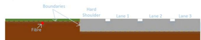
5.2.3 *Directly buried ducted fibre cable*: A duct will add to reduce the level of signal accessible on the fibre. However, a
