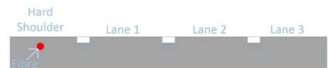
5.2.2 *Directly buried fibre cable*: Directly buried fibres, usually found at the edge of the road where the fibre cannot be slot cut into the hard shoulder, gives acoustic coupling with the ground. This method minimises the number of ground medium boundaries (road and soil) between the fibre and the traffic and therefore achieves good performance.
