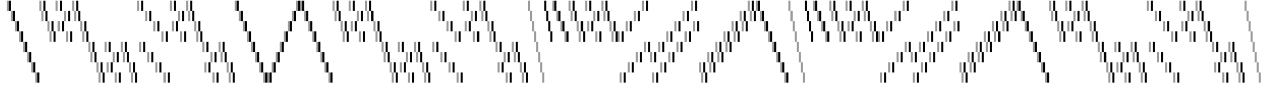
Figure 7: Visualization of our implementation’s input-independent pattern of memory access as it joins two tables of size 4 into a table of size 8. Horizontal axis is (discretized) time, vertical axis is the memory index; light shade denotes a read; dark denotes a write.
