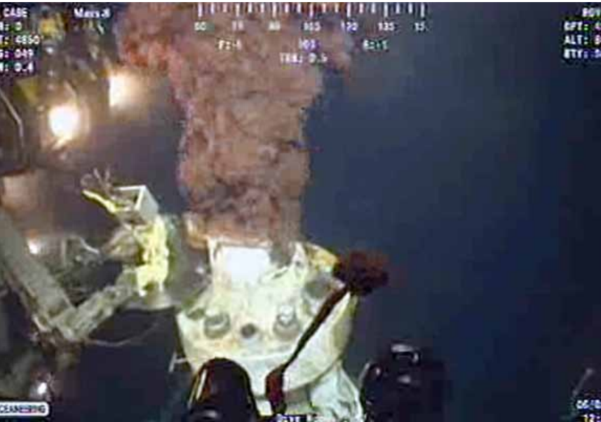
A remotely operated undersea vehicle works on the leaking riser pipe at the site of the BP oil spill, Gulf of Mexico, June 3, 2010.
