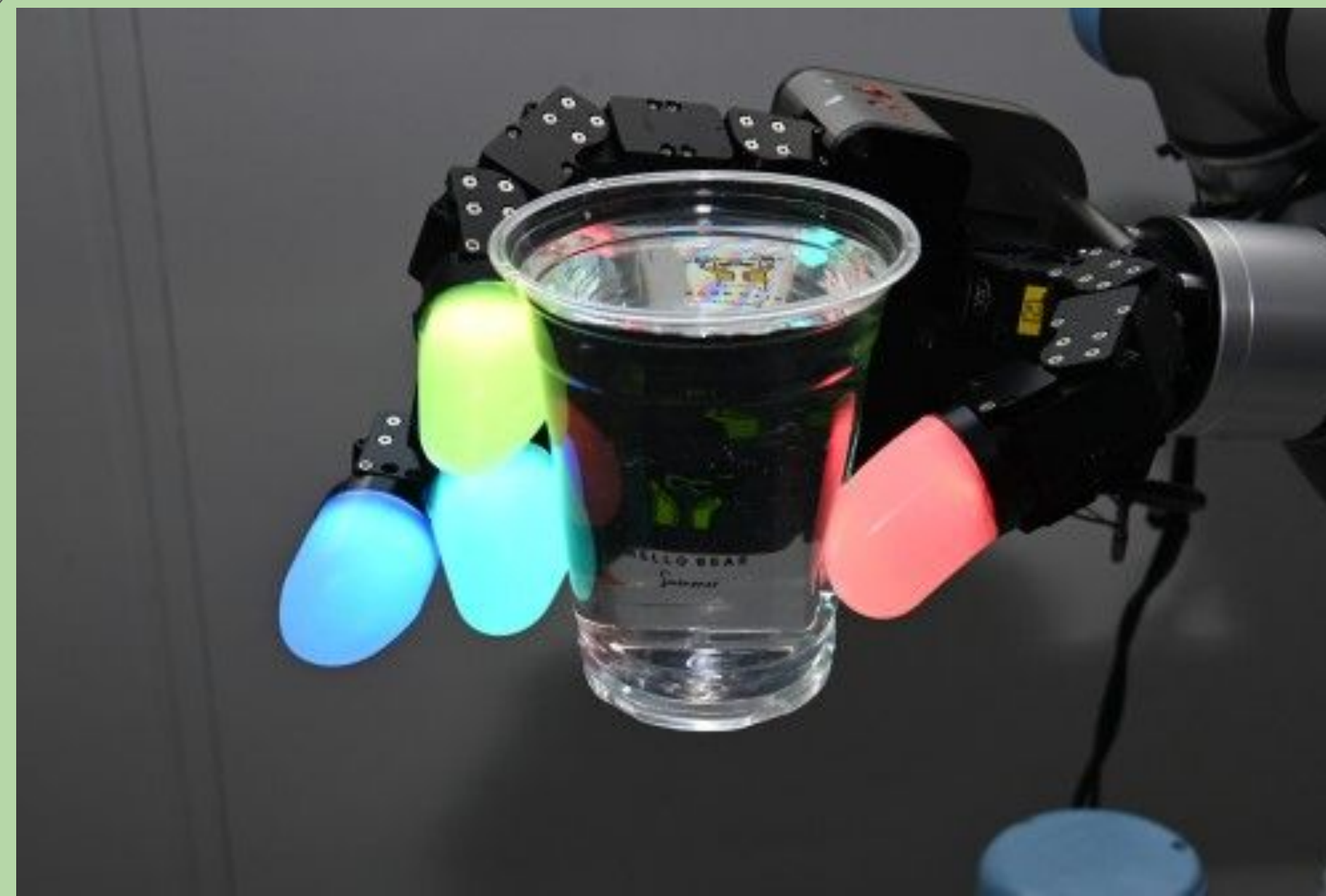
Fig 6: ETRI's omnidirectional tactile sensors (ETRI)
