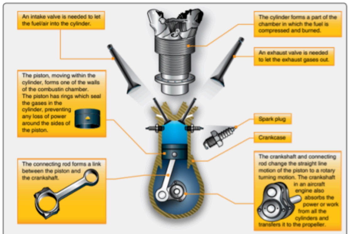
Exploded view of a cylinder of a reciprocating engine
