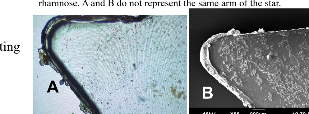
Fig 10. LM (A) mag TBD and SEM (B) pictures of PET plastics exposed to PE Tase transformed cell grown in absence of L-rhamnose. A and B do not represent the same arm of the star.
