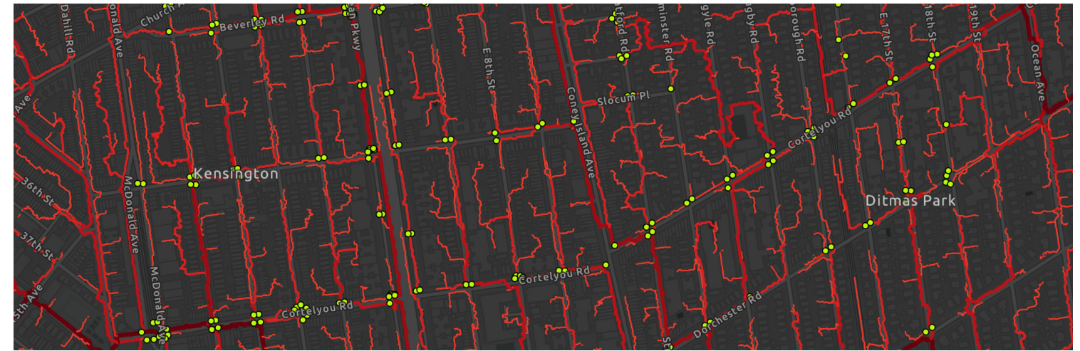
Latent streams in Kensington and Ditmas Park with catchbasins highlighted in green. Mapped by author.
