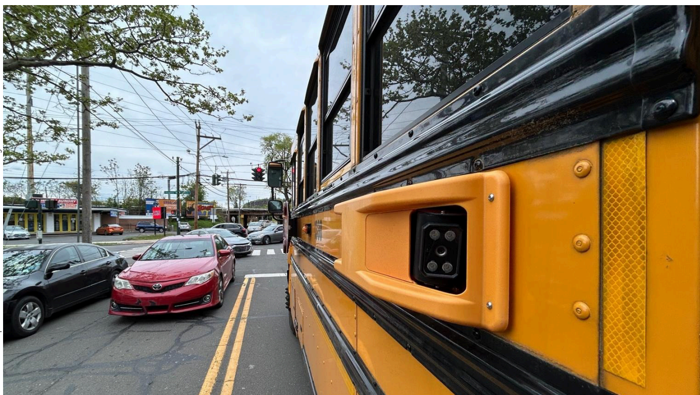
A school bus camera records vehicles that illegally pass when the bus is stopped with flashing red lights activated. The system captures violations in both directions of travel and records video and still images for review prior to citation issuance. Photo by author.
