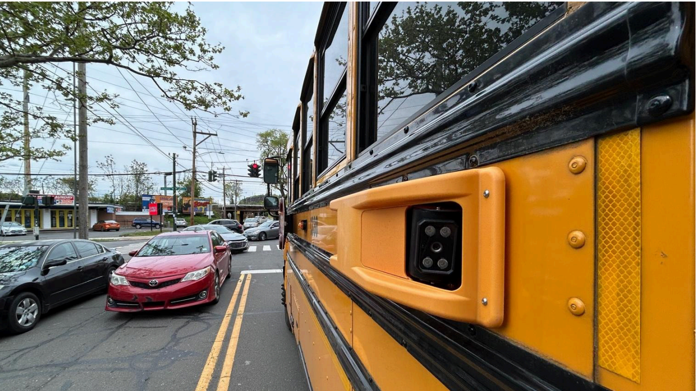
A school bus camera records vehicles that illegally pass when the bus is stopped with flashing red lights activated. The system captures violations in both directions of travel and records video and still images for review prior to citation issuance. Photo by author.
