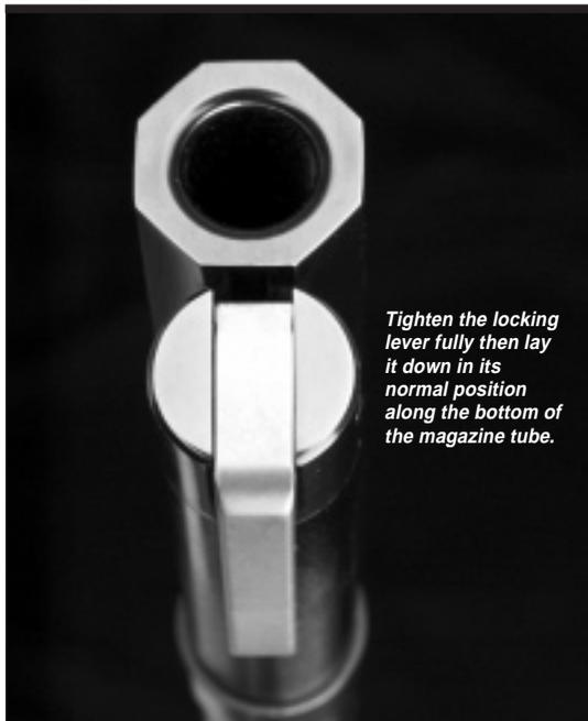
*Tighten the locking lever fully then lay it down in its normal position along the bottom of the magazine tube.*
