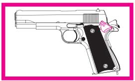
The **hammer safety** is engaged when the hammer is cocked and the thumb selector lever is switched into the up position. When the hammer is not cocked, this safety cannot be engaged, however, it can be engaged if the hammer is half-cocked.
