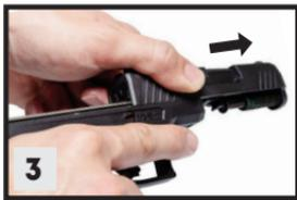
3. While pointing the pistol in a safe direction, pull the **trigger** and push the **slide** forward away from the **grip** to separate it from the **slide**.
