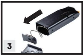
1. Use a **punch** to press in on **magazine spring seat/clip** as shown in figure 1.
