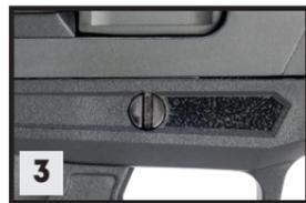
3. The **slide** should be mounted on the **frame** and pulled fully to the rear. Engage the **slide catch**. Using a flat head screwdriver, rotate the **take down pin** clockwise 1/4 turn until the slot is positioned vertically. Release the **slide** by pulling down on the **slide catch**.
