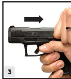
3. Hold the pistol with one hand keeping your finger away from the trigger and on the **Indexing pad/(RMP)**. With the other hand pull the **slide** to its rear limit and release it, the **slide** will go forward under **recoil spring** pressure and will insert one cartridge into the **chamber**.
