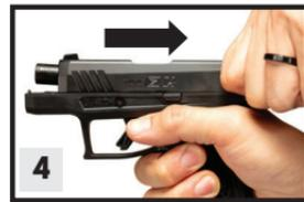
4. With the **magazine** removed, you should cycle the **slide** several times, to insure that the **barrel / slide / frame** fit together properly.
