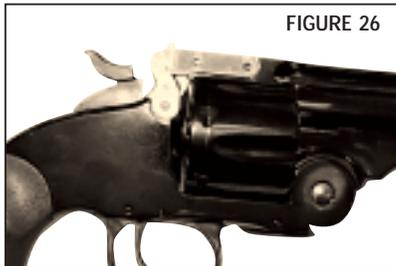
**NEVER ATTEMPT TO OPEN OR CLOSE THE BARREL/FRAME WITH THE HAMMER IN THE "AT REST" POSITION. FAILURE TO FOLLOW THIS WARNING WILL CAUSE DAMAGE TO YOUR FIREARM.**
