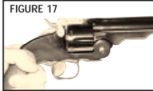
With your fingers outside of the trigger guard and a firm hold on the grips, place the thumb of your non-shooting hand on the hammer spur. Draw the hammer fully rearward until it is cocked as shown in (Figure 16). The revolver will now fire when the trigger is pulled.
