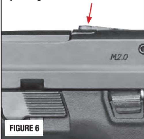
Tactile loaded chamber indicator flush with top of slide when no round is present in the chamber
