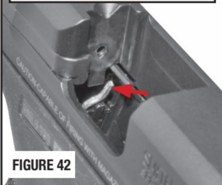
View from the top - through the ejection port - with slide locked open. The sear deactivation lever has been lowered.
