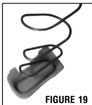
**CAUTION:** Verify that the end of the spring is fully inserted and seated into the recess on the bottom of the magazine follower. (Figure 19)
