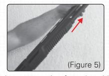
Remove the pump action forend upside parallel to the barrel. (Figure 5)
