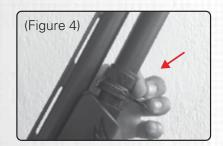
To remove the forend turn the magazine cap part counter-clockwise and remove the part. (Figure 4)
