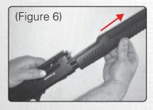
Remove the forend by holding the back the bolt action. (Figure 6)
