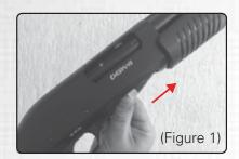
Release the loading port and push cartridges into the magazine tube. Repeat until magazine tube is full. (Figure 1)
