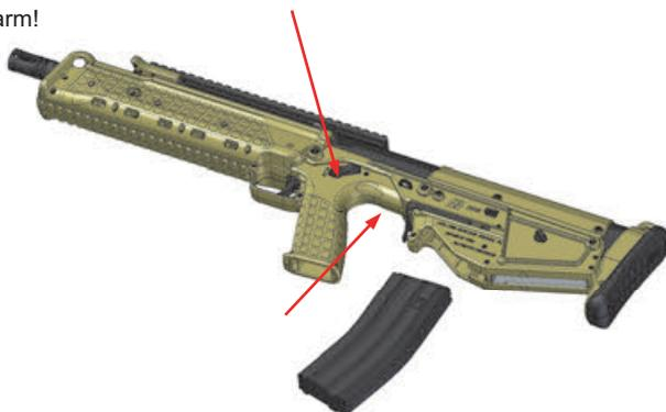
Insert a loaded magazine into the well behind the pistol grip. Make sure it is engaged by the magazine catch. Unfold the operating handle and pull it all the way back. Release the handle and let it go forward by its own power.
