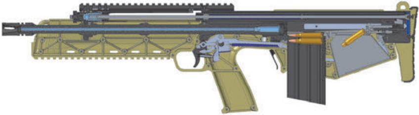
Two integral MIL-STD-1913 Picatinny rails, located above the barrel and on the handguard, come standard with the RDB™ for mounting compatible accessories. The RDB™ maintains a center of gravity over the grip assembly to facilitate ease of handling and balance.
