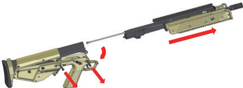
4. Pull the bolt carrier out of the barrel assembly.
