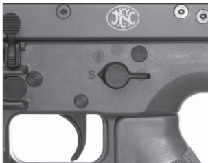
Safety shown in the on safe position.
