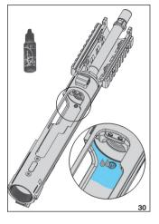
CAUTION: Do not apply excess oil. Accumulation of oil attracts dirt and dust, which can interfere with the functioning and reliability of the firearm.
