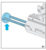
Insert the sling swivel properly oriented.
