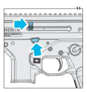
2) with no magazine in the pistol, retract the bolt while pressing up on the bolt catch to lock the bolt in the open position.
