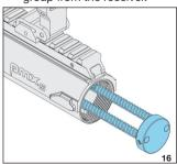
Align the cocking handle with the hole in the receiver and remove it by pulling it outwards.
