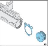
8. Remove the recoil spring group from the receiver.
