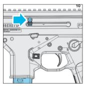
Notice: The bolt will be released when pulled to the rear if a LOADED magazine is inserted.
