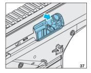
If the spent case or the cartridge have been ejected and the chamber is empty, release the cocking handle to feed a new round.
