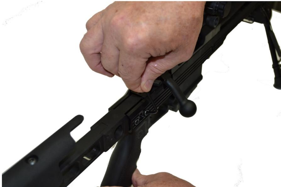
***Removing the Buttstock***
