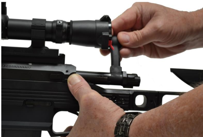
*Removing the Bolt Assembly*
