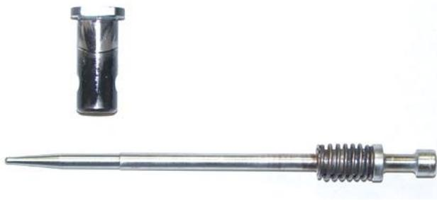
9. Inspect the cam pin for cracks or chips.
