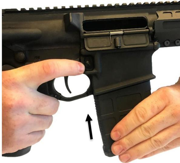
3. Pull down on the magazine slightly to make sure that it is locked in place.
