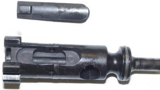
5. Press the ejector in repeatedly to remove accumulated brass shavings from the ejector hole and assure the ejector moves freely. Lubricate it generously.
