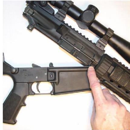
**⚠ CAUTION: TO AVOID DAMAGE TO THE EJECTION PORT COVER, CLOSE THE EJECTION PORT COVER BEFORE THE RECEIVERS ARE JOINED.**
