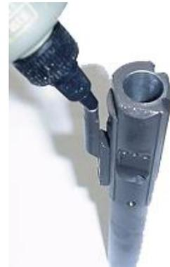
**Note:** Carbon in the groove at the bottom of the gas cylinder in the carrier cannot accumulate enough to become a problem. Efforts to remove it cause more damage than leaving it. Avoid the instinct to over-clean your rifle.
