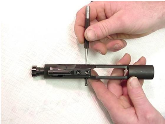
4. Move the bolt assembly forward to the unlocked position and remove the firing pin retaining pin. This can be done by either pushing it from right to left with a pin punch or pulling it from the “loop” side. Do not open or close the split end of the firing pin retaining pin.
