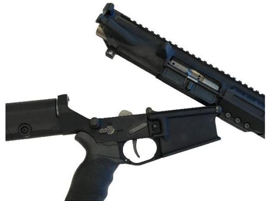
**⚠ CAUTION: EXCESS FORCE CAN SEVERELY DAMAGE THE RECEIVER. ALWAYS SUPPORT BOTH UPPER AND LOWER ASSEMBLIES WHEN DISASSEMBLING**
