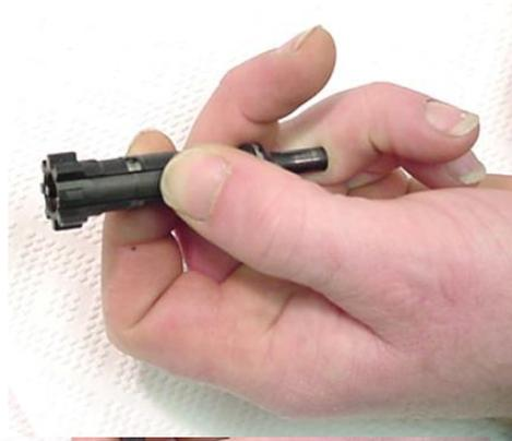
10. Use a punch or dummy round to remove the extractor pin.
