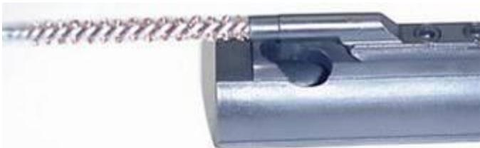
2. Clean the bolt carrier key with a worn bore brush dipped in solvent and dry with a pipe cleaner.
