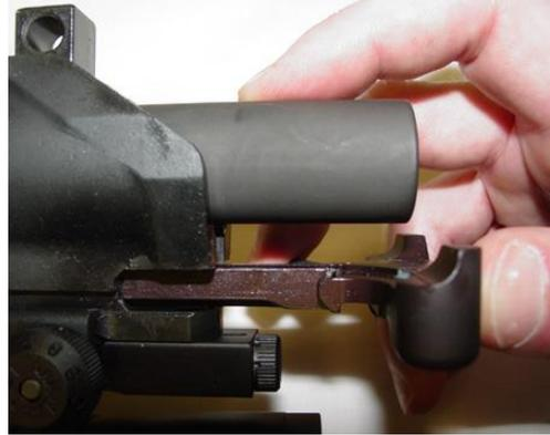
12. Reinstall the handguard over the barrel assembly pushing it until the upper receiver and the top tail on the handguard are fully contacted and aligned.
