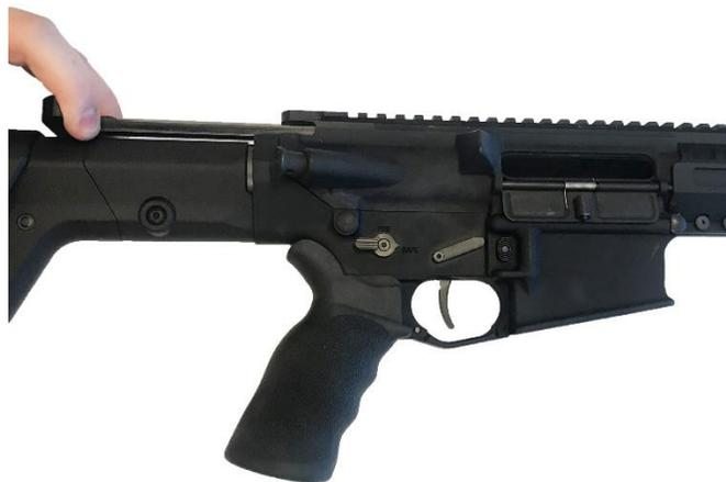
2. Push the magazine up into the receiver until the magazine catch engages and holds the magazine.
