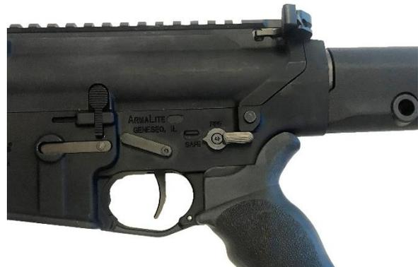
**2. Remove the magazine by depressing the magazine catch button and pulling the magazine down.**
