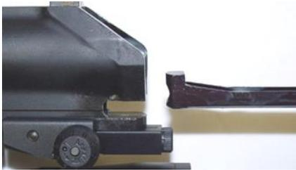
3. Pull the charging handle back aligning the tabs on the charging handle with the cut outs on the inside of the receiver and bring it down to remove it.
