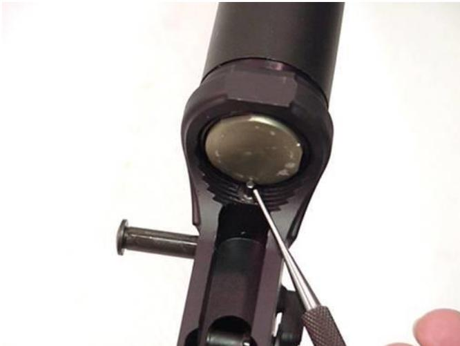
1. Cock the hammer with your thumb. Push in the buffer and depress the buffer detent to release the buffer.
