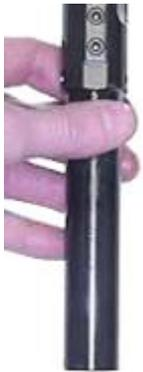
8. Turn the bolt carrier assembly up and try to shake out the firing pin. The firing pin must not fall out.
