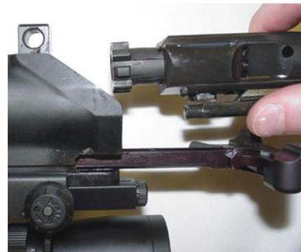
11. Push the charging handle assembly and bolt carrier assembly together into the upper receiver.
