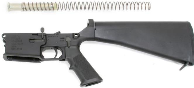
3. Clean the buffer, operating spring, and inside lower receiver with a swab dipped in solvent.
