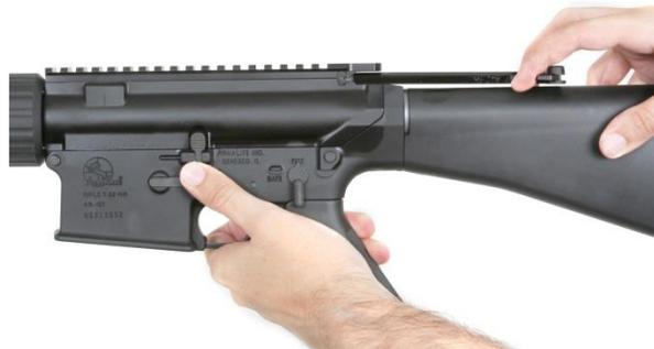
3. Place the safety on “SAFE”. Squeeze the trigger. *The trigger should not fall.*
