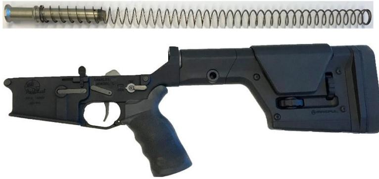
2. Remove the buffer and the operating spring
