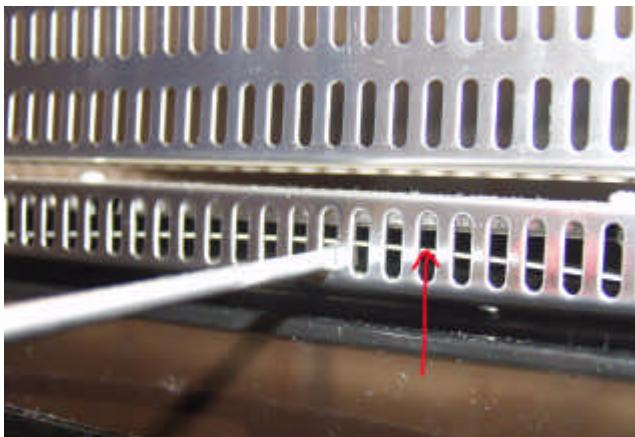
The solution is to use something to lift the curved steel sheet free of the top of the oven and spray in some graphite grease powder on both sides where the contact with the top of the oven box is made. This is VERY messy stuff - if you spill it on the floor remove if promptly with a little Jiff or similar.
