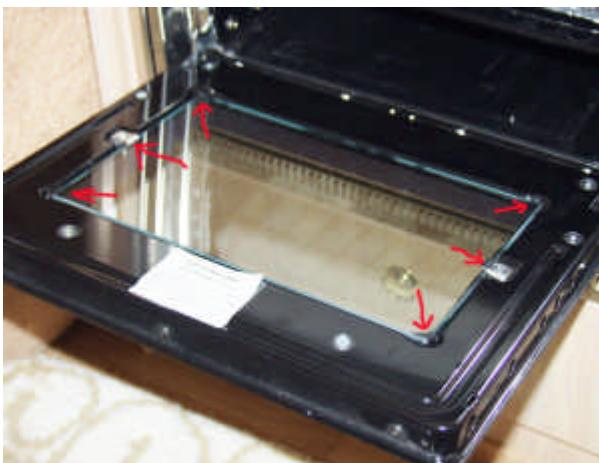
Remove the glass and place a small amount of Silicone designed for high temperature applications under each corner and under each bracket and replace the glass. DON'T use ordinary Silicone..... This stuff is hard to find - try an industrial bearing supplier.
