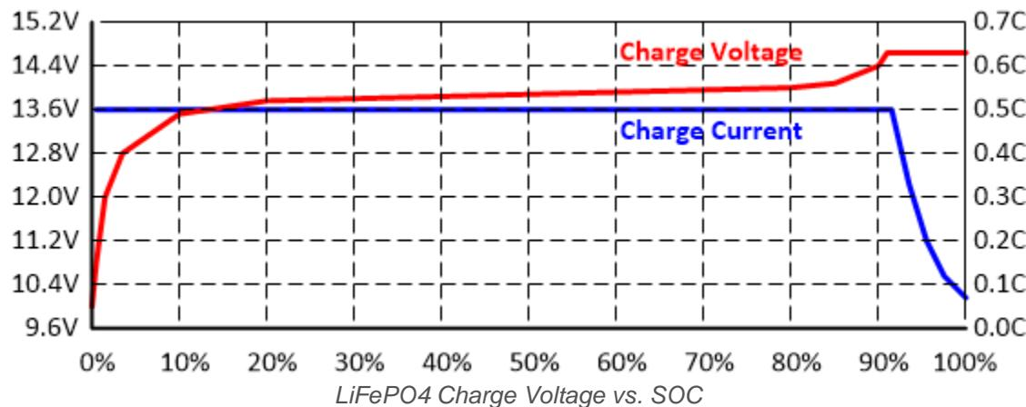
Shown in the graph is a charge rate of 0.5C, or half of the Ah capacity, in other words for a 100Ah battery this would be a charge rate of 50 Amp. The charge Voltage (in red) will not really change much for higher or lower charge rates (in blue), LFP batteries have a very flat Voltage curve.
