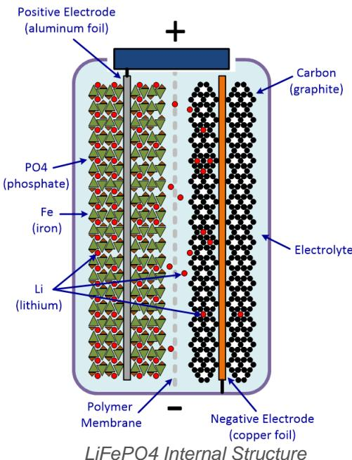
Lithium-ion batteries move ions, in this case lithium ions, from the negative to the positive electrode when discharging, and back again when charging. The diagram shows what goes on inside. The little red balls are the lithium ions that move back and forth between the negative and positive electrodes.
