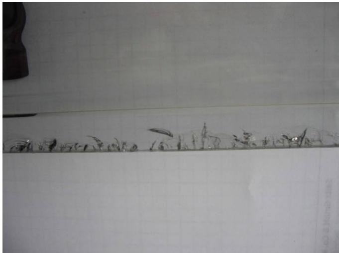
Cracks on lower edge of an S4 window.
