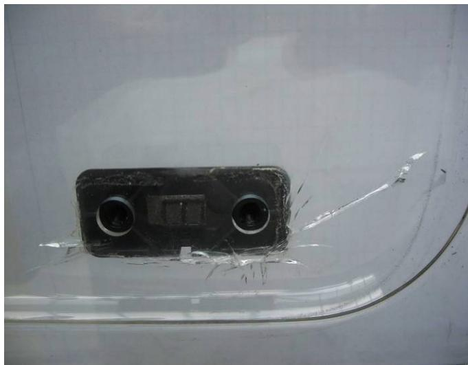
Cracks on the inner pane in the area of the anchorage of the catch.
