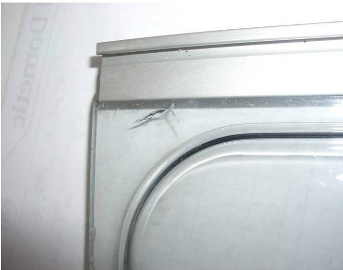
Cracks form starting from under the hinge profile of an S4 window.
