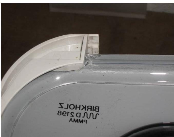
Cracks start to form in hinge profile area and corner of a C1 window pane.
