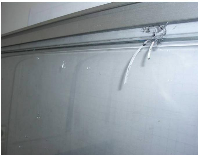
Big cracks in the hinge profile area.
