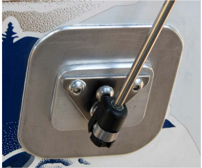
Lower Stainless Steel Pivot Ball Installation on a 2005 Aliner
