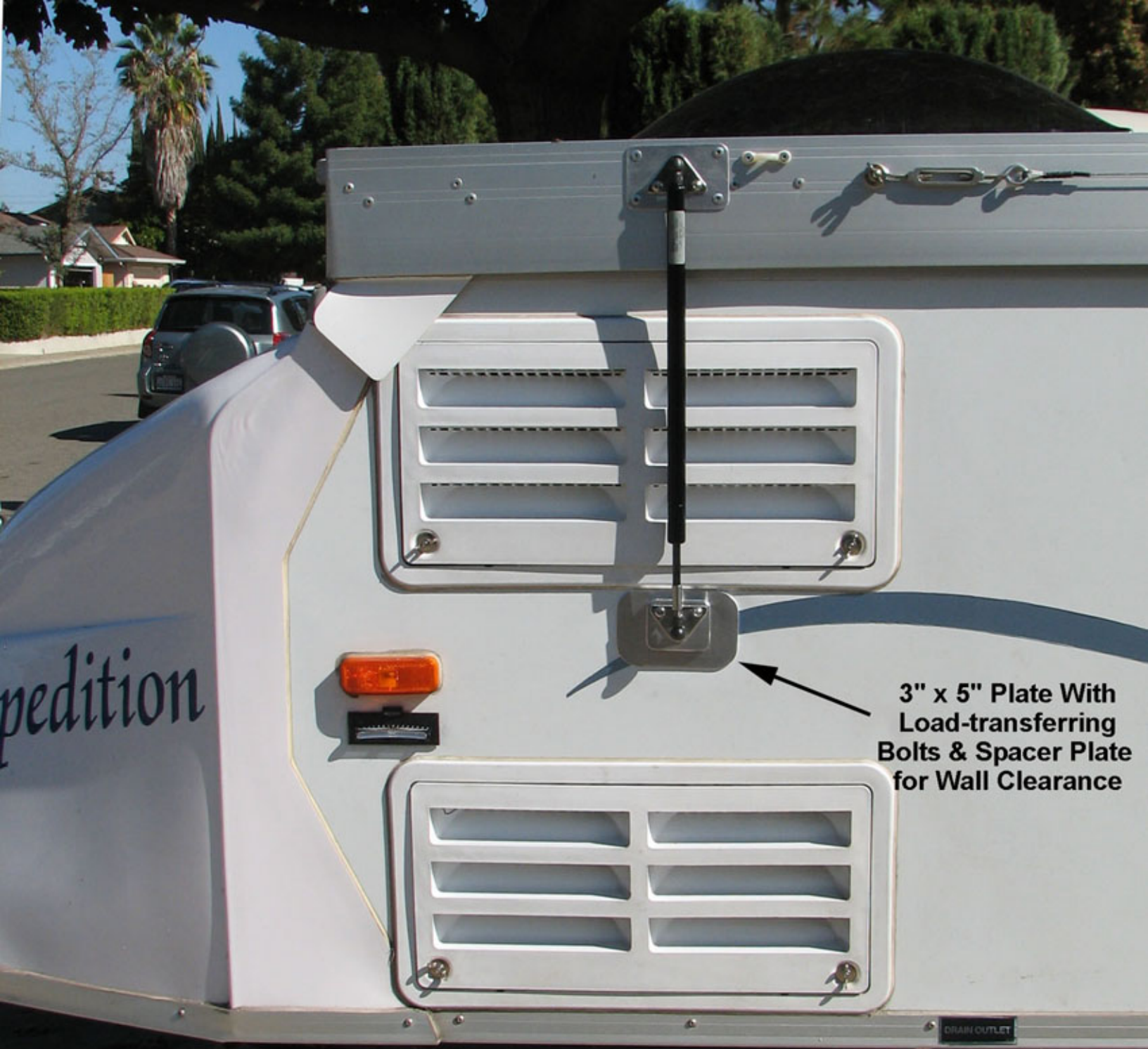
26" Gas Spring Added Between Refrigerator Vents
