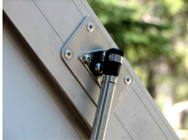
Upper Stainless Steel Gas Spring Mounting Plate on a 2005 Aliner
