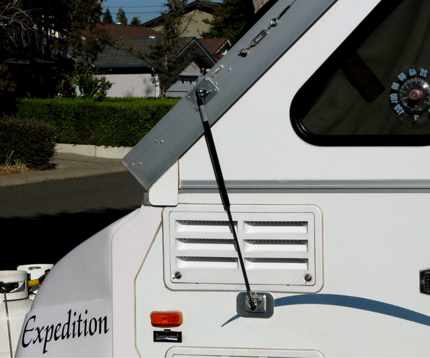
26" Gas Spring Added to the Refrigerator Area
