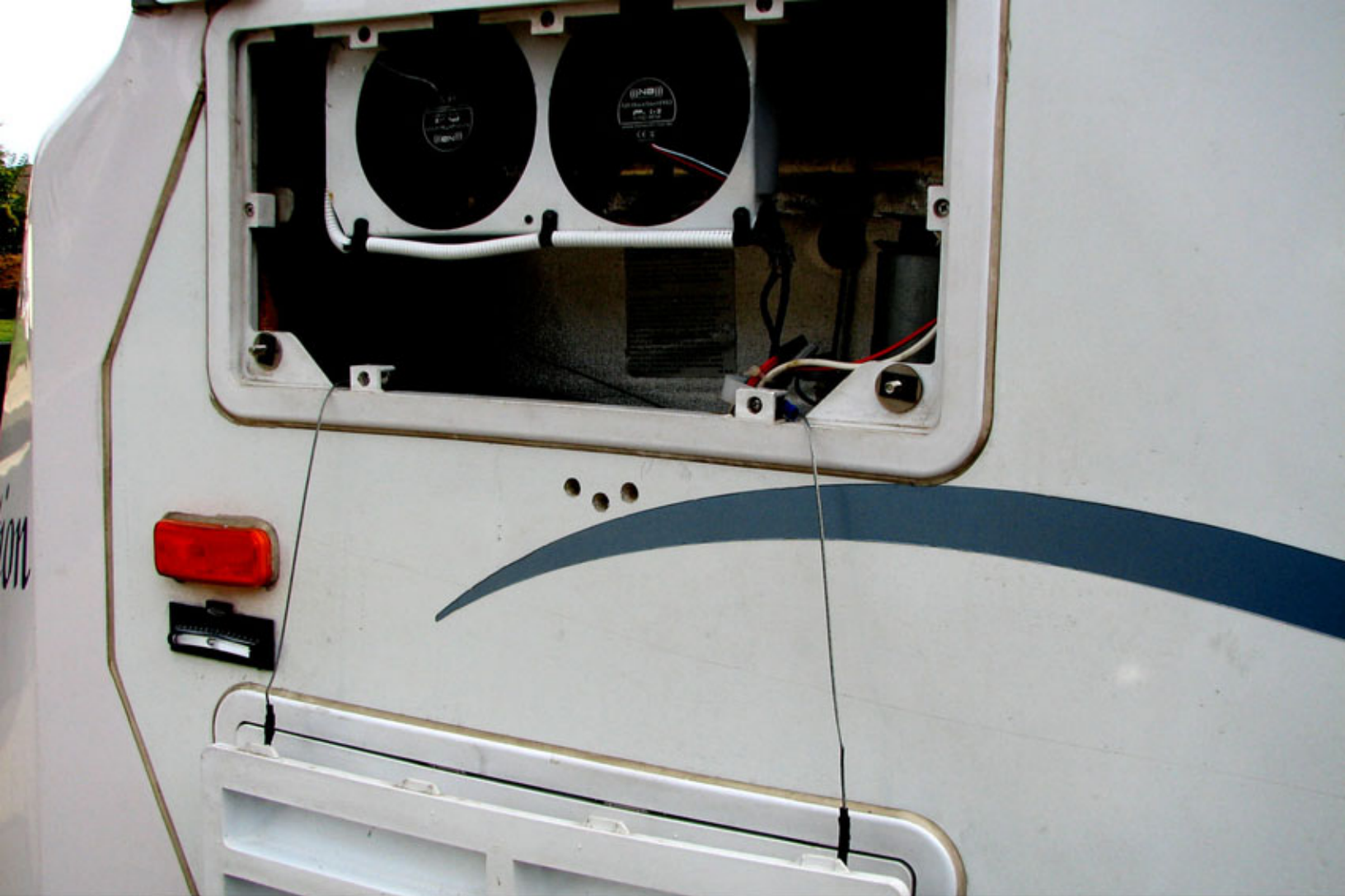
Holes Drilled for Gas Spring Lower Pivot Ball Mounting System
