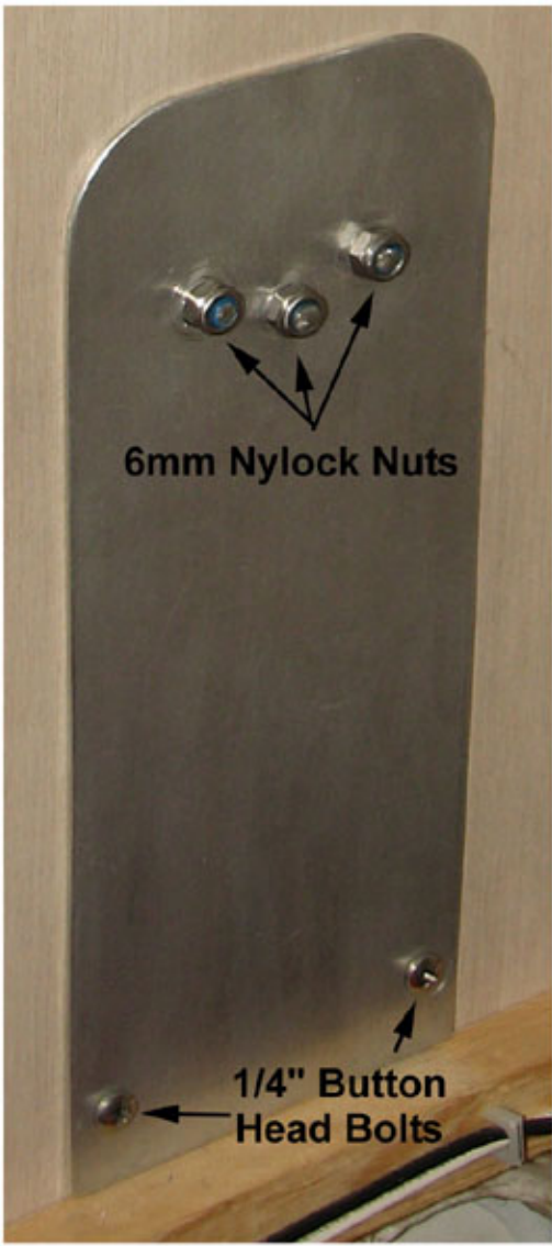
Interior Load Transferring Plate Installation
