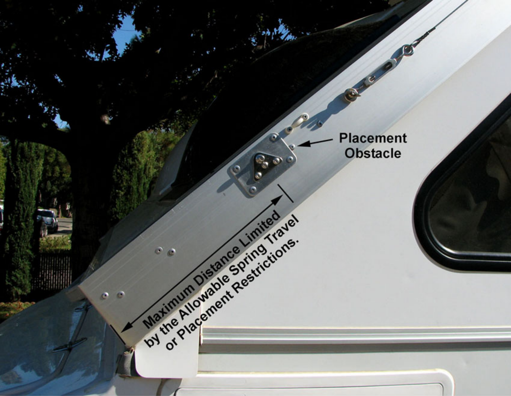
Installation of the Upper Pivot Ball Mounting System
