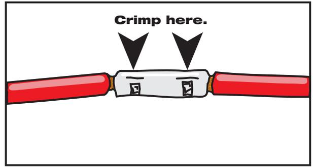
Crimp both wires to the butt splice using indent type crimpers.
