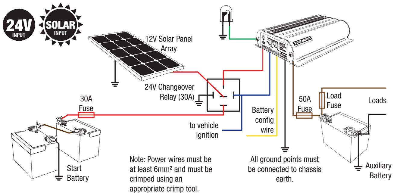
Figure 2.6 - Standard setup for a 24V Start Battery & 12V Solar array
