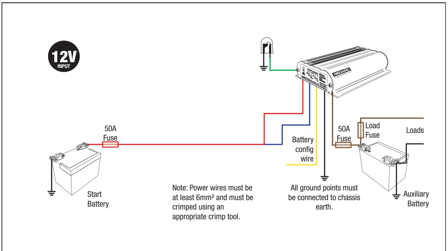
Figure 2.2 - Standard setup for a 12V Start Battery
