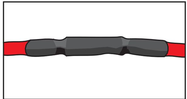
Wait for the butt splice to cool, slip heatshrink over the joint and heat.
