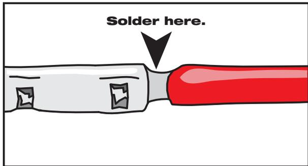
Solder the wires to the butt splice. Ensure that a good connection is made.
