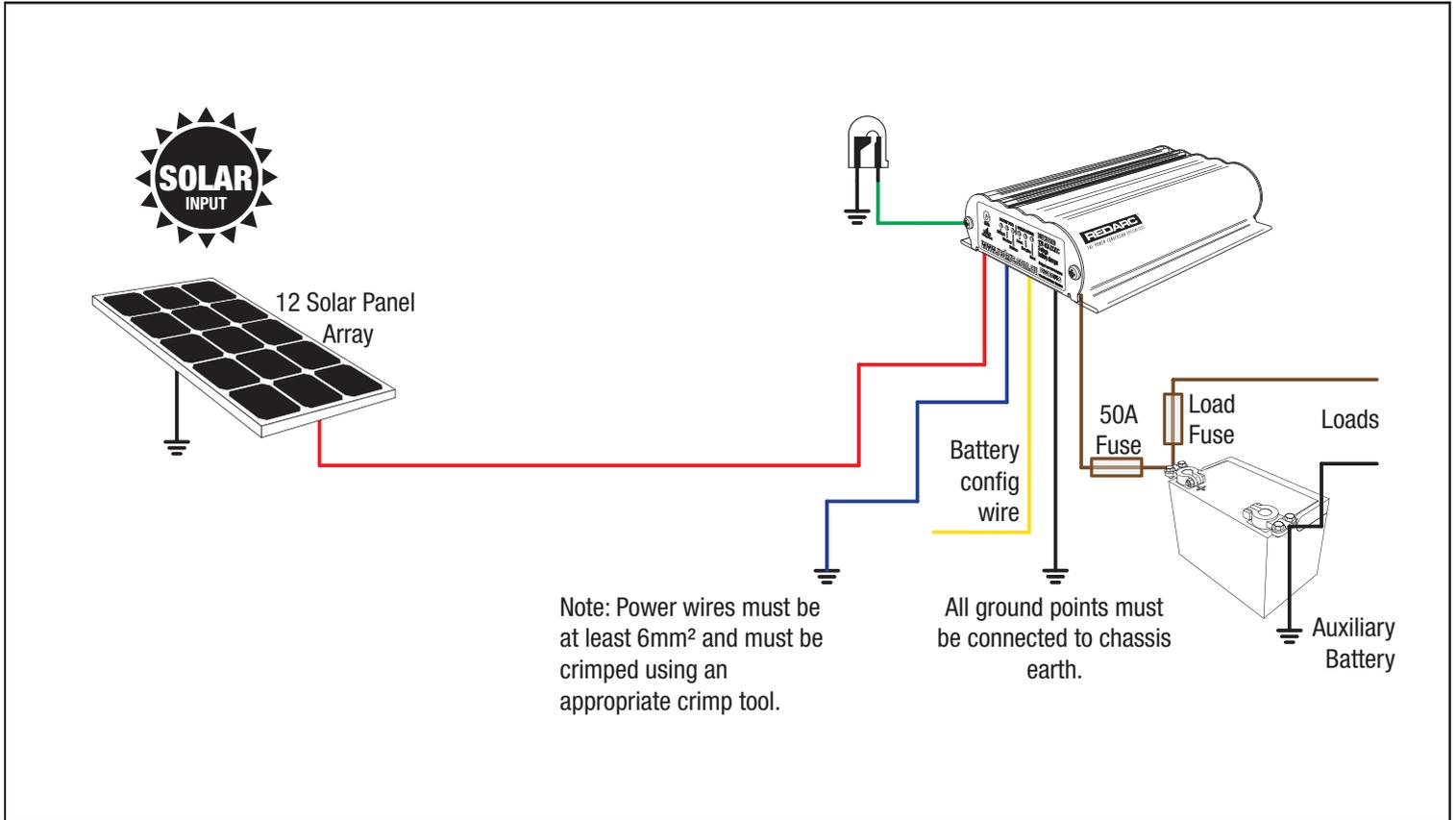
Figure 2.3 - Standard setup for a 12V Solar array
