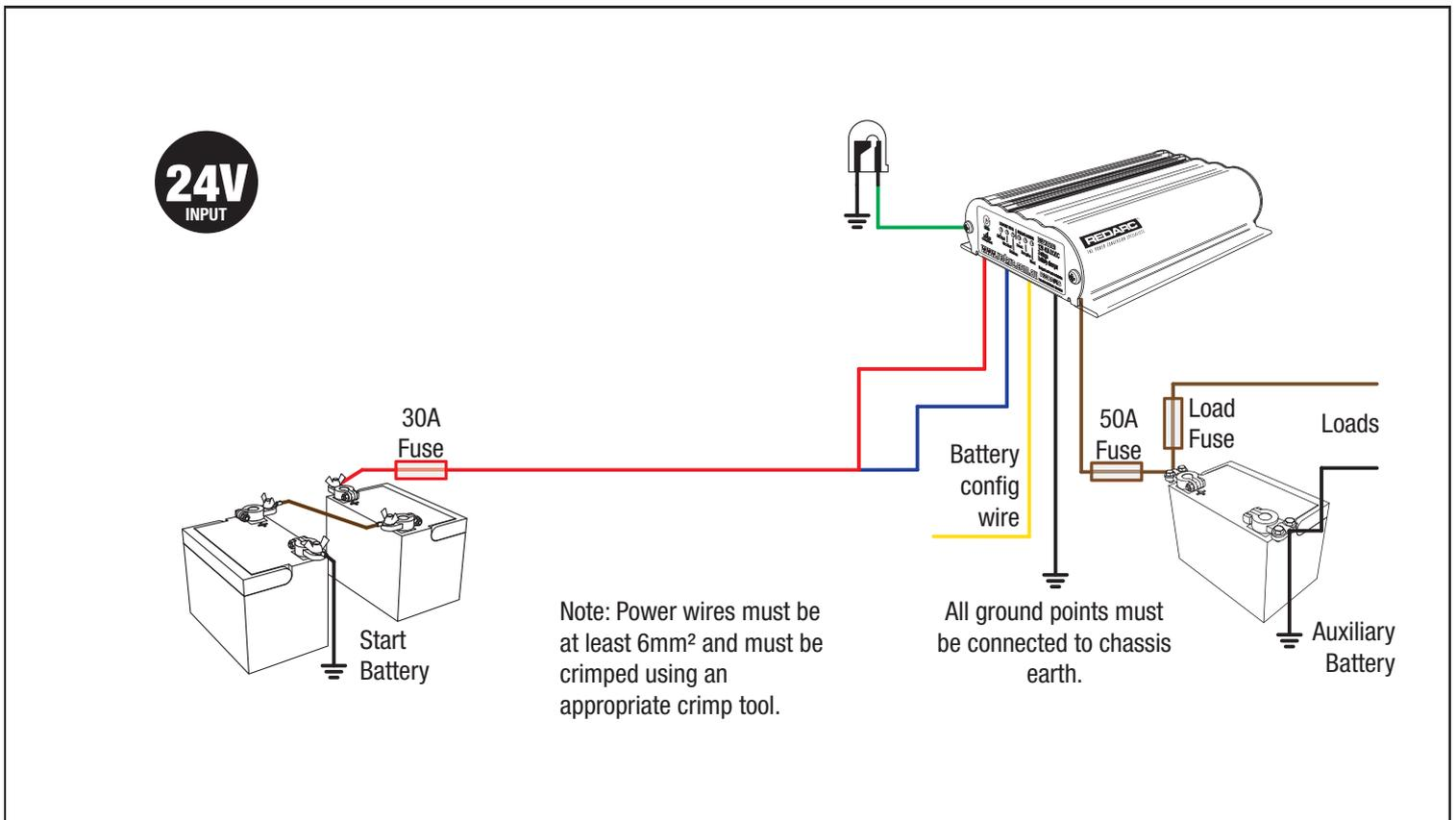
Figure 2.4 - Standard setup for a 24V Start Battery
