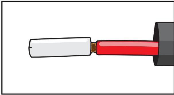
Slip heatshrink over wire and insert wires into butt splice. Keep heatshrink away from joint until after soldering is complete and has cooled.
