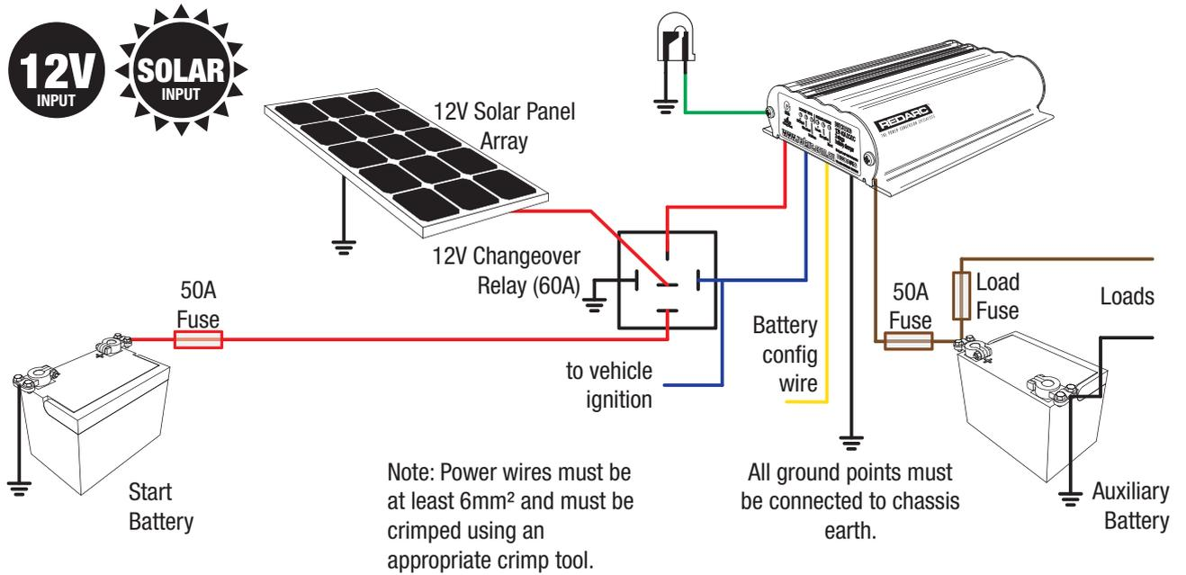
Figure 2.5 - Standard setup for a 12V Start Battery & 12V Solar array
