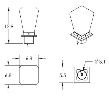
Mounting Method: Mounts Directly To Post
