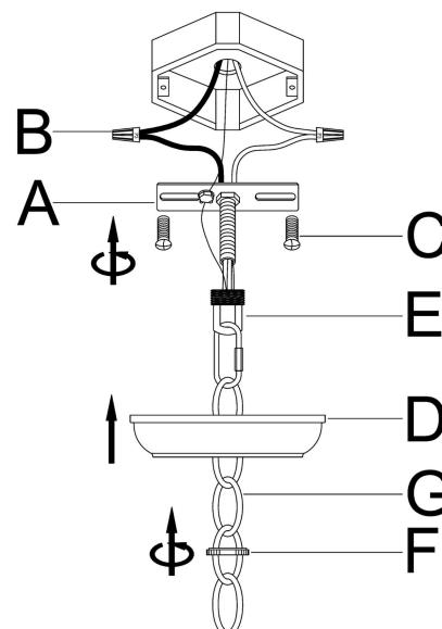
**Step 5:** Attach the Canopy(D) to the junction box and fix it by turning the Canopy Nut(F) clockwise.
