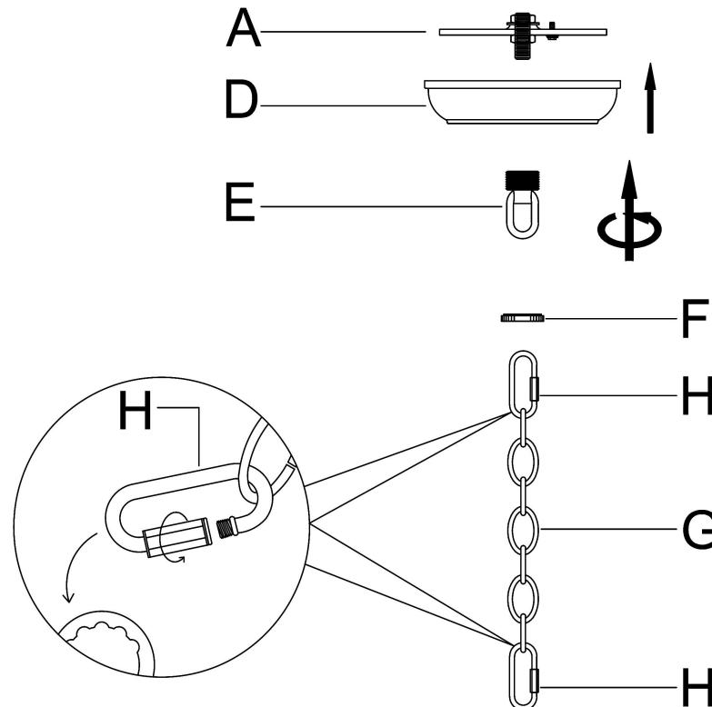
**Step 1:** Unpack all parts from cartons carefully. Place the Canopy (D) onto the Hanging Loop (E).
