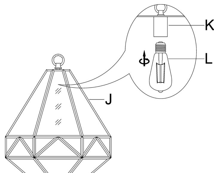
**Step 6:** Insert the bulbs (L) into the Sockets(K).
