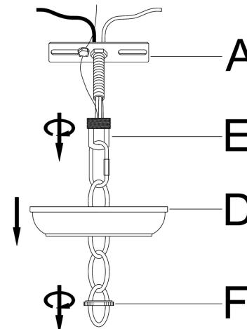
**Step 4:** Install the Mounting Plate(A) to the junction box with Mounting Screw (C). Separate the Mounting Plate(A) from the Canopy(D) by turning the Canopy Nut(F) anti-clockwise.
