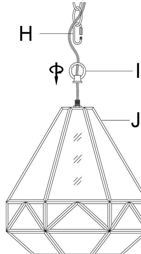
**Step 2:** Thread Fixture Loop (I) to Shade (J) of the nipple. Attach the Closable Link (H) onto the Fixture Loop (I).
