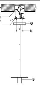
**Step 5:** Attach the Canopy(G) to the junction box and fix it by turning the Canopy Nut(K) clockwise.
