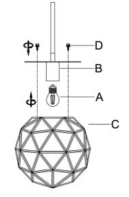
**Step 6:** Insert the bulbs (A) into the Sockets(B).Fix the Sockets (B) to the Lamp body(C) with Final Screw(D).
