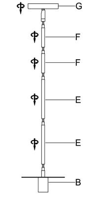
**Step 2**:Screw the Long Stem (E) and Short Stem (F) to the Socket (B). Make sure to feed the branch wires of the fixture through the stems during assembly. Remove or add stems to adjust the height. Then screw the canopy (G) to the stem.
