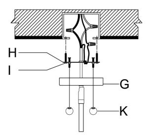
**Step 4:** Fix the Mounting Plate(H) to the junction box with Mounting Screw (I).
