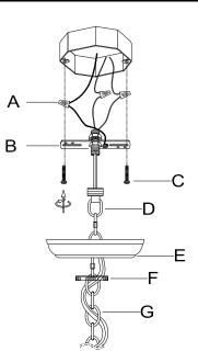
**Step 4:** Attach the Mounting Plate (B) onto the junction box by inserting two Mounting Screws (C) and turning clockwise till tight.
