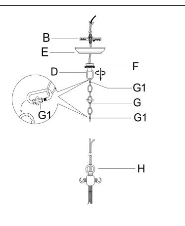
**Step 2**:Screw the Chain(G) to the Hanging Loop(D) and the loop of the Socket Assembly(H) with Closable link/cap (G1) as diagram.
