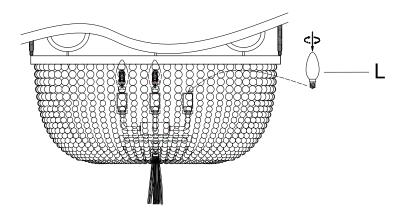
**Step 5:**Insert the bulb(L) into the socket.DO NOT EXCEED THE SPECIFIED WATTAGE.
