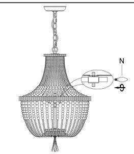
Step 6: Insert the bulbs (N) into the Sockets.
