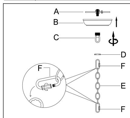
**Step 1:** Unpack all parts from cartons carefully.Place the Canopy(B)onto the Hanging Loop(C).
