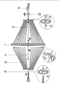
**Step 2:**Insert one end threaded portion of the Long Tube(H) into the tube upper the Lamp Body (I). Insert one end threaded portion of the Short Tube(J) into the tube underneath the Lamp Body (I). Place the Lamp Body(I) above the top thread portion of the Long Tube(H)and fix it by turning the Fixture Loop(G) clockwise. Insert the bottom threaded portion of the Short.
