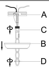
**Step 4:** Install the Mounting Plate(A) to the junction box with Mounting Screw (M). Seperate the Mounting Plate(A) from the Canopy(B) by turning the Canopy Nut(D) anti-clockwise.
