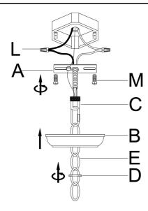
**Step 5:** Attach the Canopy(B) to the junction box and fix it by turning the Canopy Nut(D) clockwise.
