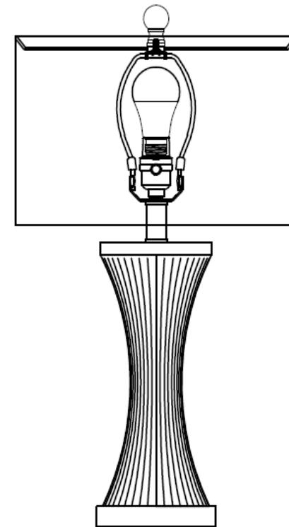
**Step1:** Insert the Harp (D) into the Saddle (B). Put the shade (E) on the Harp(D), then tighten the Finial (F) into the Harp (D), Insert the bulb (G) into the socket (C). Be careful not to twist the power cord and tighten securely.
