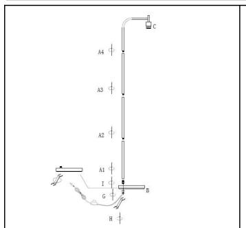
**Step1**:Make sure all parts could be aligned before assemble .Do not rotate lamp body too hard avoid base screw broken.Separate the hexagon nut(J) and Parts(I) from lamp base(B) by using wrench(H).
