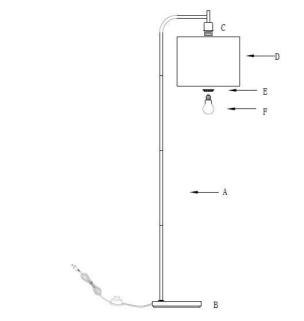
**Step2:** Put the shade(D) on the socket (C). Screw the ring(E) on the socket (C). Insert the bulb(F) into the socket(C).
