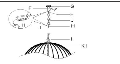
**Step 2:**Screw the Chain(J) to the Hanging Loop(F) and the Fixture Loop (I) with Closable link/cap (H)as diagram.
