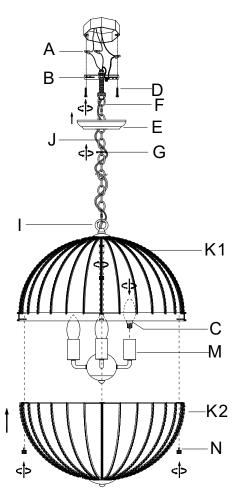
Step 5: Attach the Mounting Plate (B) onto the junction box by inserting two Mounting Screws (D) and turning clockwise till tight.Slide the Canopy (E) upward along the chain(J) till the ceiling surface. Fix the Canopy(E) by rotating the Canopy Nut(G)clockwise to engage it with the threaded portion of the Hanging Loop (F) until secure. Do not over tighten this nut.Insert the bulbs(C) into the sockets(M) until secure. DO NOT EXCEED THE SPECIFIED WATTAGE.
