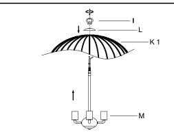
**Step 1:** Unpack all parts from cartons carefully.Insert the power cord of the Socket Assembly(M) to the Top Frame(K1),Metal Cover(L),Hanging Loop(I). Then fix the Top Frame(K1) by turning the Hanging Loop(I)clockwise till tight.
