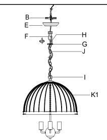
**Step 3:** Weave the 2 wire power cord and bare ground wire through every other loop to the top of chain(J),center holes of Hanging Loop(F)&Canopy(E)&Mounting Plate(B) as diagram.Insert the threaded tube of the Mounting Plate(B)into the center hole of the Hangling Loop(F),rotate the Mounting Plate(B) clockwise till tight.Slide the Canopy Nut(G) then the Canopy(E) to the end of the Chain(J).
