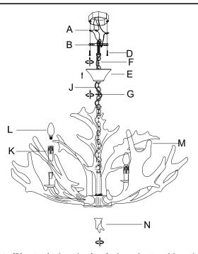
**Step 4:**Attach the Mounting Plate (B) onto the junction box by inserting two Mounting Screws (D) and turning clockwise till tight. Slide the Canopy (E) upward along the chain (J) till the ceiling surface. Fix the Canopy(E) by rotating the Canopy Nut(G) clockwise to engage it with the threaded portion of the Hanging Loop (F) until secure. Do not over tighten this nut.
