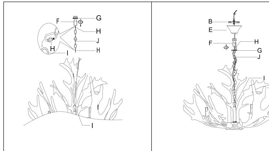
**Step 1:** Unpack all parts from cartons carefully. Screw the Chain(J) to the Hanging Loop(F) and the Fixture Loop (I) with Closable link/cap (H) as diagram.
