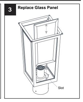
Reverse the above steps to reinstall the glass holder and the cage.
