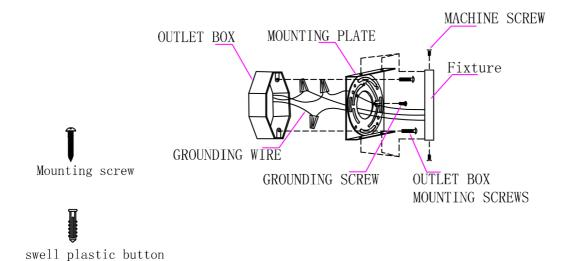
CAUTION :DISCONNECT POWER DURING INSTALLATION 1.) If you are replacing an existing fixture, disconnect and remove the old fixture. Expose the supply wiring from the outlet box.
