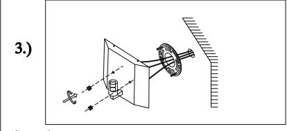
Step.3: Screw finials (D) onto mounting bracket (A)
