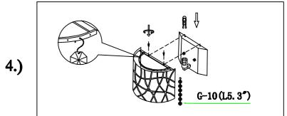
Step.4: Fix the shade (H) with the canopy by provided screws, and install G9 bulbs (F) and hang Crystal strands(G)
