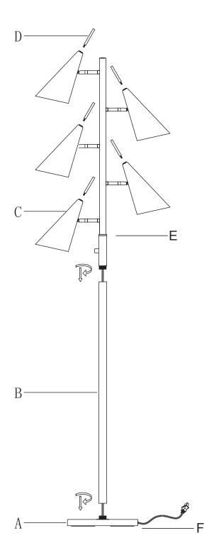
1.Screw pole(B) clockwise into base(A) to tighten. Then get remaining slack of the power cord out carefully from point(F).
