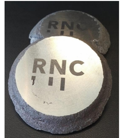
Ferro-nickel puck produced from Dumont concentrate
