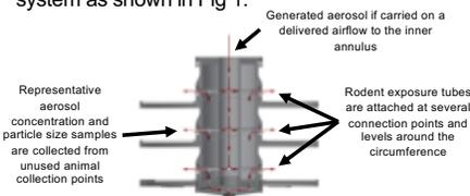
Figure 1, Inhalation Dosing. Aerosol is generated as required and delivered via a central annulus from which each animal, restrained in a restraint tube, receives individual and identical aerosol exposure. Exhaust is collected from the tubes and removed using the outer annulus. This mechanism allows for a consistent delivery of aerosol with no filtering or rebreathing by animals at different points on the system
