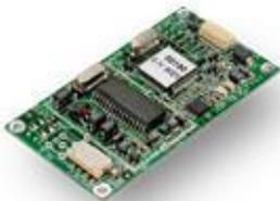
The *OTI Interno* (SCI 6100 OEM) global original equipment manufacturer, or OEM, reader module with integrated antenna is a compact and cost-effective contactless card reader board, designed for easy integration into mass transit validators and terminals.
